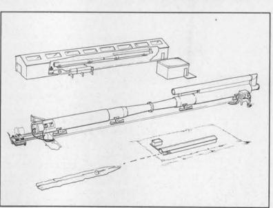
AIR GUN test installation for Area III as the artist conceives it is shown here. At the top is a cutaway drawing of the building to house the gun. In the center is the gun showing the two 16-inch naval cannons flanged together. At the left is the breech end of the gun containing the compressed air chamber. Lower drawing shows an open end shot with the projectile fired into the target area. Construction bids were opened this month for the three buildings to house the test facility.
